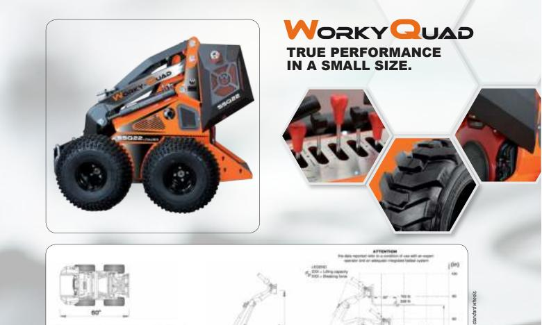
**SSQ 22 LOADER** Engine: Honda HGX690 - Displacement 688 cc Number of cylinders: 2 Start up: Electric Revolutions per minute: 3600 Cooling: air cooled Fuel: petrol Fuel tank capacity: 4,4 gal Drive system: Hydrostatic 4WD wheel motors Hydraulic tank capacity: 8,8 gal Standard tyres: 22x11.00-8 All Trac Steering: Skid steering Kerb weight: 1390 lbs
